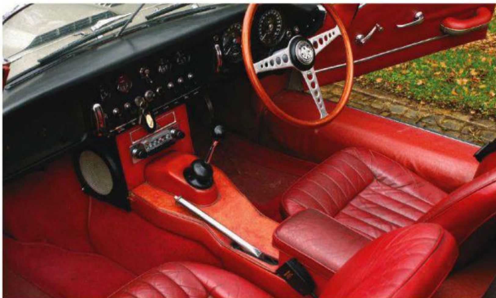
Left Armchair comfort, huge twin dials, hinge-forward instrument panel, bold switches, wood-clad wheelrim and useless handbrake.
